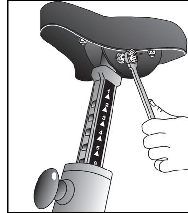
**Diagram 9: Loosen nut to adjust seat tilt**
