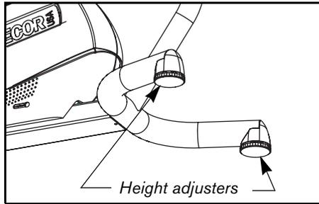
To remove any side-to-side movement, ask your assistant to tip the unit on its side so that you can locate the two height adjusters on the rear crossbar.
