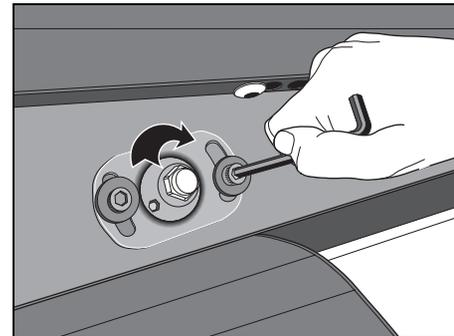
**Diagram 11: Loosen the two adjustment screws**
